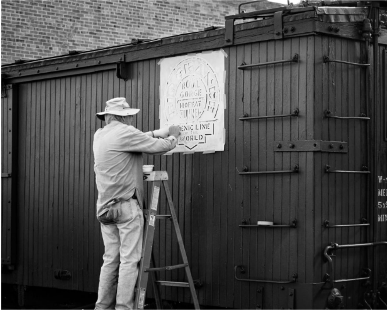
One of the Friends of the C&T volunteers paints new lettering on this boxcar, the same way they would have done 100 years ago.
